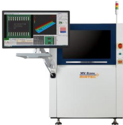
The new high speed, high performance 3D AOI Machine boasts 15 mega pixel CoaXPress camera technology, as well as advanced eight phase color lighting system. The machine includes a ten micron/pixel precision telecentric compound lens design, integrated ten mega pixel side-viewer camera system, and a precision closed loop AC servo drive motor system.
